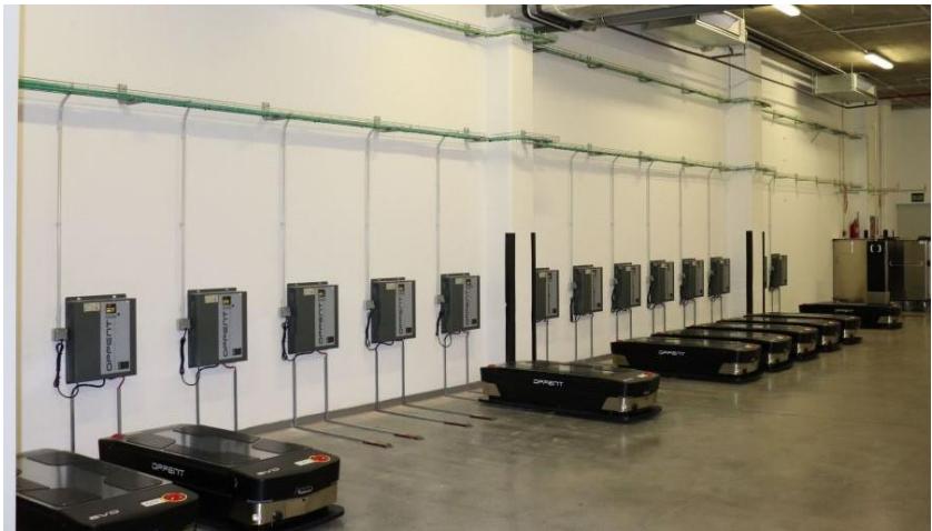
The mobile robots charging stations provided by Oppent for the CAUSA in Salamanca
